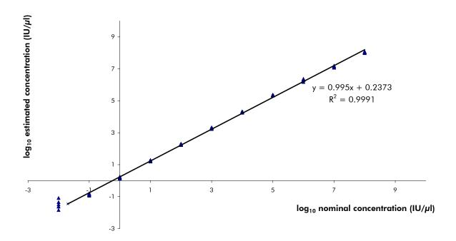
Figure 2. Linear Range of the artus HBV RG PCR Kit. Calculation of the linear range. The straight line was determined by a linear regression of the  $\log_{10}$  calculated concentrations with the  $\log_{10}$  nominal concentrations. The equation of the regression line is included in the figure.
