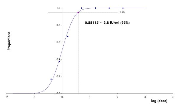
**Figure 1. Probit analysis: HBV (Rotor-Gene 3000).** Analytical sensitivity in consideration of the purification (QIAamp DSP Virus Kit, QIAGEN) of the *artus* HBV RG PCR Kit on the Rotor-Gene 3000.
