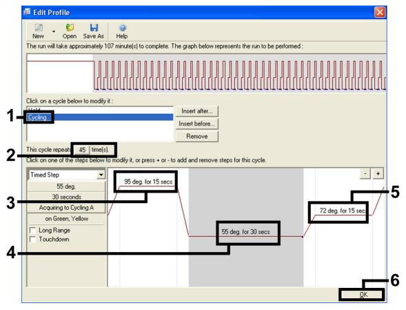
**Figure 8. Amplification of the DNA.** Note that, on the Rotor-Gene 3000, the software will define the fluorescence dyes as "FAM/Sybr, JOE".
