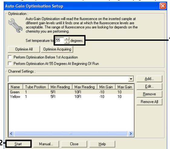
**Figure 9. Adjusting the fluorescence channel sensitivity.** Note that, on the Rotor-Gene 3000, the software will define the fluorescence dyes as "FAM/Sybr" and "JOE".
