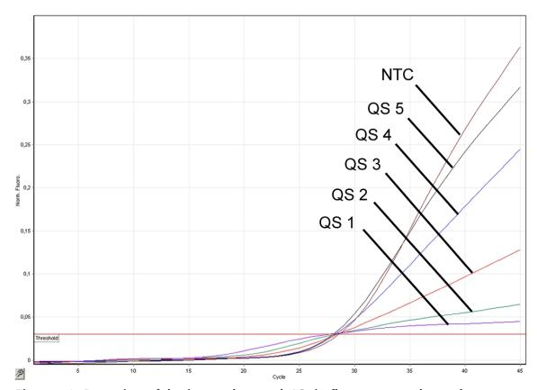
Figure 12. Detection of the internal control (IC) in fluorescence channel Cycling Yellow with simultaneous amplification of the quantitation standards (HBV RG/TM QS 1–5). NTC: No template control (negative control).
