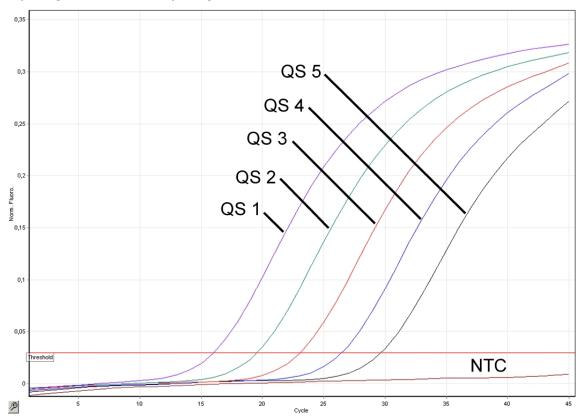
Figure 11. Detection of the quantitation standards (HBV RG/TM QS 1–5) in fluorescence channel Cycling Green. NTC: No template control (negative control).
