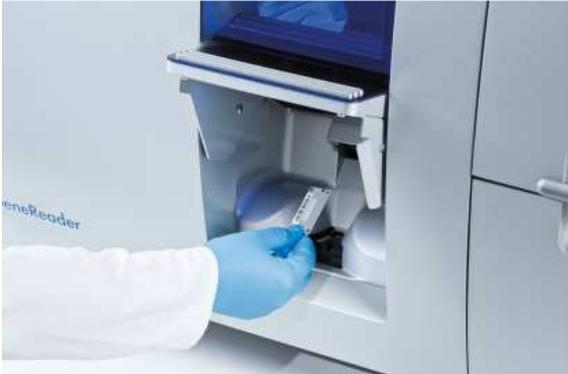
**Figure 4. Loading the Flow Cell of GeneReader.**
