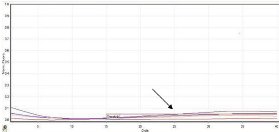
**Figure 3. Example of a linear increase in fluorescence in an NTC tube.** The arrow indicates linear increase in fluorescence in a NTC tube.
