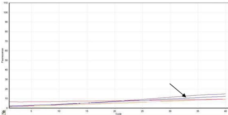
**Figure 4. Raw fluorescence data in NTC well.** The arrow indicates linear amplification in an NTC well.
