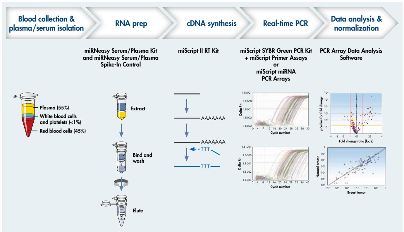
Figure 4. miScript PCR System workflow.
