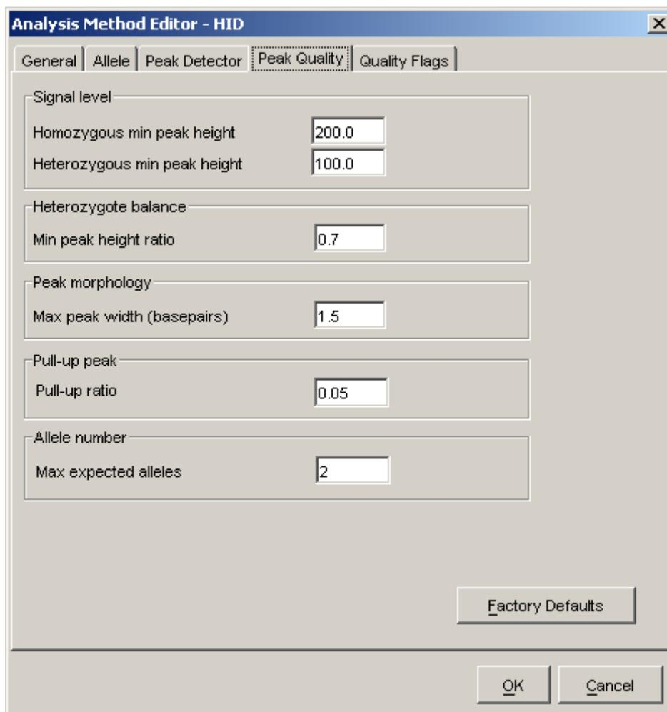
**Figure 8. The Peak Quality tab. Peak Quality is used to adjust peak quality parameters.**
