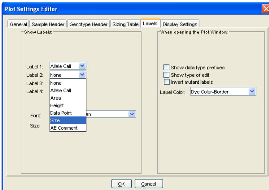
The Labels tab is used for setting which labels are displayed for each peak in an electropherogram.
