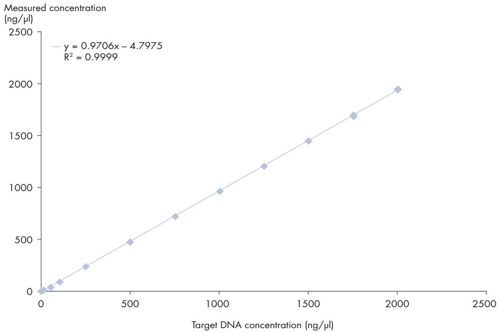
**Figure 2. Excellent measurement linearity of QIAxpert.** The spectrophotometry data were plotted against the target concentration. The data demonstrate outstanding linearity for samples with concentrations up to 2000 ng/μl or 40 OD ( $A_{260}$ , 10 mm), respectively. The calculated regression coefficient is >0.999.
