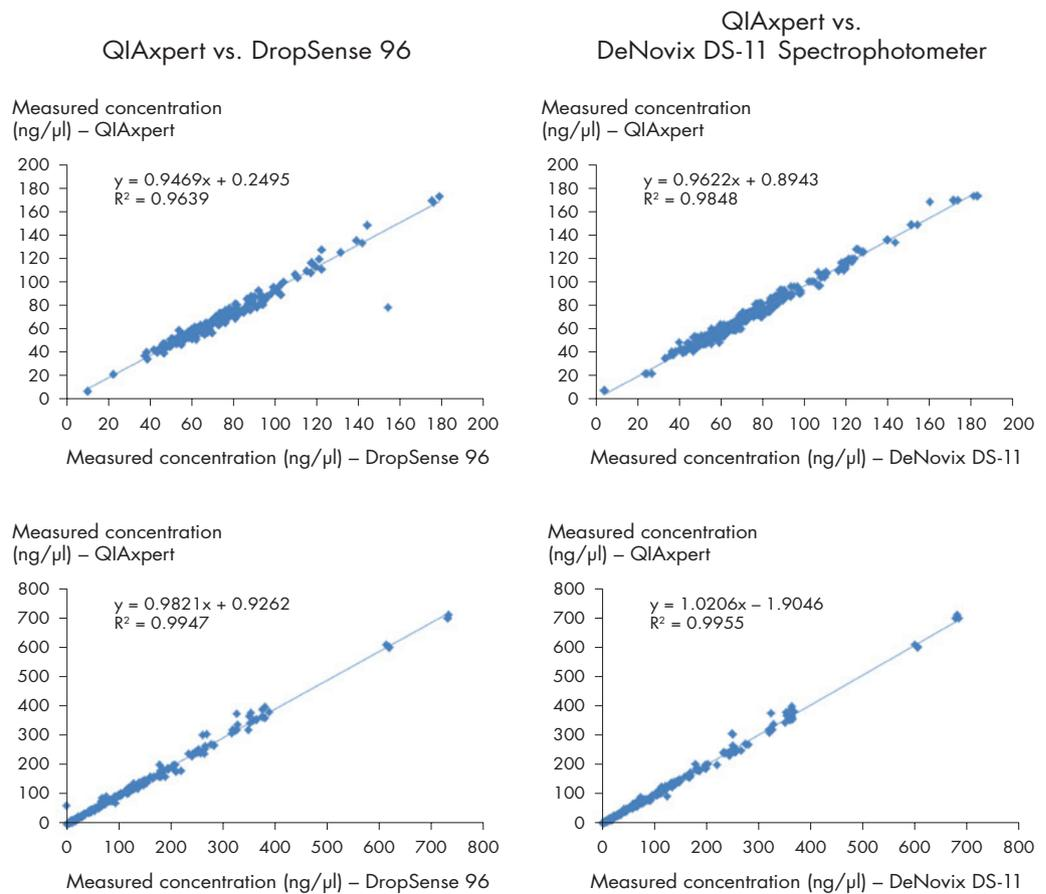
**Figure 4. Reliable measurement performance of QIAxpert for field DNA and RNA samples.** QIAxpert, DropSense 96 and the DeNovix DS-11 Spectrophotometer were employed to measure concentration of field DNA and RNA samples. Right: Analyses of the DNA (top) and RNA (bottom) samples with the DeNovix DS-11 Spectrophotometer and QIAxpert yielded highly comparable results, indicated by the regression line slopes being close to 1. Left: Similarly, results with the DropSense 96 were comparable.
