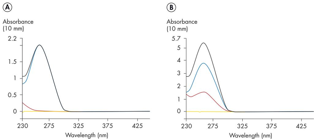
To test the linearity of the system, we prepared samples of various concentrations ranging from 1 to 2000 ng/ $\mu$ l from a commercial solution of pure salmon sperm DNA. Each dilution was measured 5 times using 2  $\mu$ l samples pipetted onto QIAxpert slides. The results demonstrate high concordance of the quantifications made on the QIAxpert system with the target concentrations over the complete range of concentrations measured (Figure 2).
