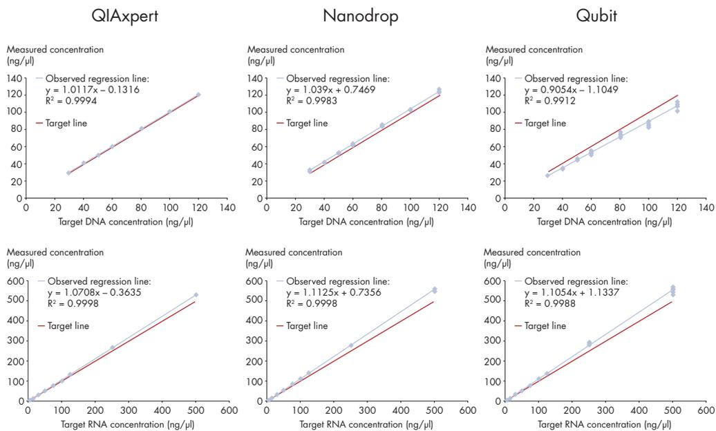
**Figure 3. Superior linearity of concentration measurements for commercial DNA and RNA samples using QIAxpert.**
