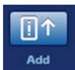
Use the **Add** command to load flow cells during a run in staggered mode once the first cycle of sequencing is complete, and prior to 24 hours after the run has started. Refer to Section 5.2.3 for more information.
