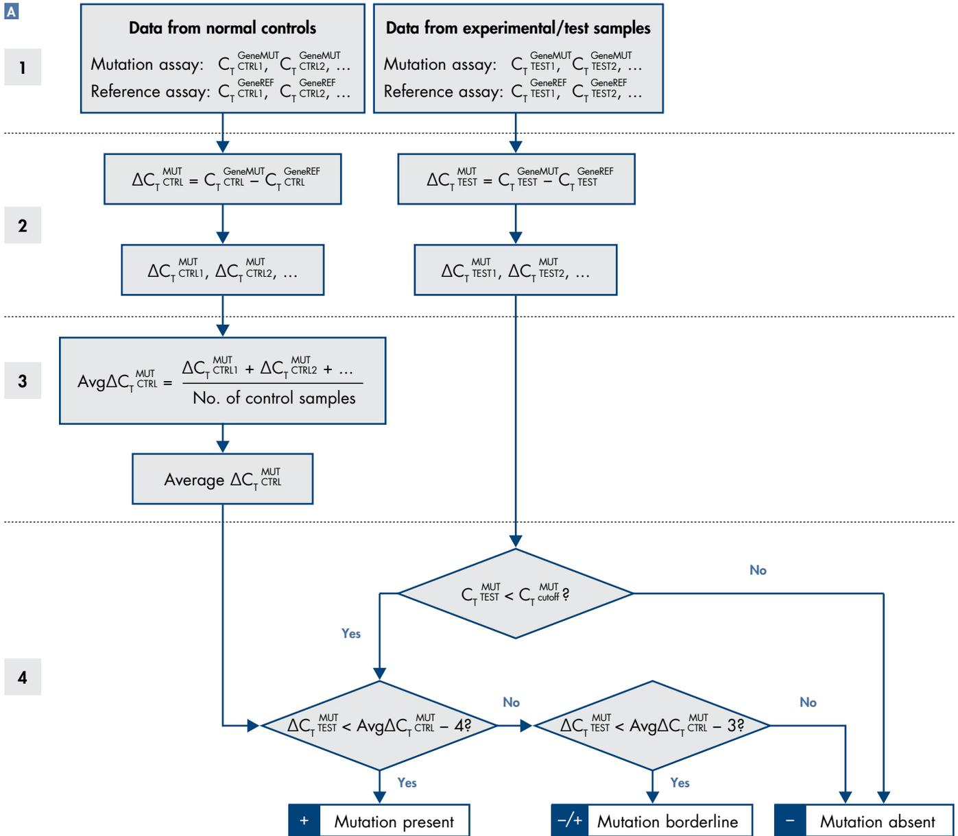
**Figure 5A. Data analysis workflow for the  $\Delta\Delta C_T$  method.**
