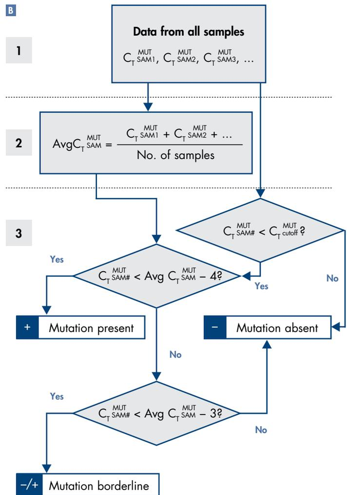
**Figure 5B: Data analysis workflow for the average  $C_T$  method.**
