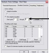
Set the baseline from cycle number 2 through two cycle values before the earliest visible amplification.
