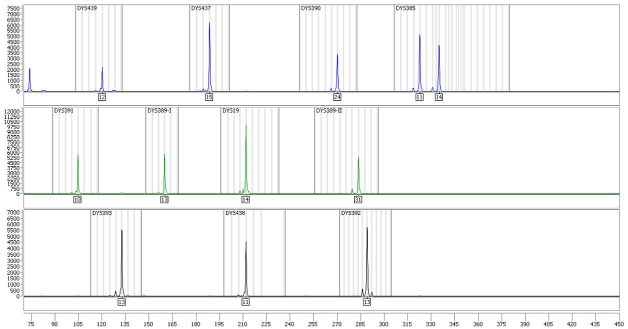
**Figure 4. Electropherogram of the Investigator Argus Y-12 QS Kit using 500 pg Control DNA 9948.** The Quality Sensor (QS) is shown at 74 bp. Analysis was performed on an Applied Biosystems 3500 Genetic Analyzer with the DNA Size Standard 550 (BTO). Allele assignment was performed using Investigator IDproof Software.
