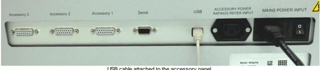
USB cable attached to the accessory panel.
