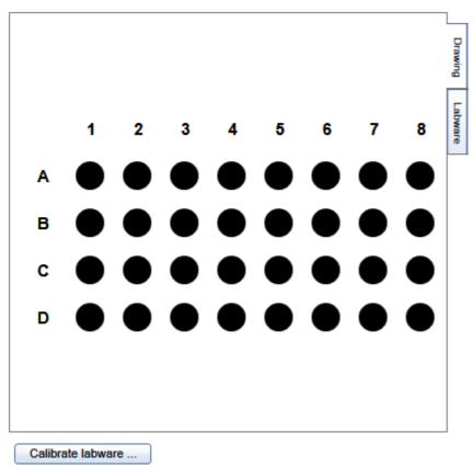
Adapter: 32 x 1.5 ml Flip-Cap Tapered-Base Tubes Labware: 1.5 ml tapered tube (QIAGEN)
