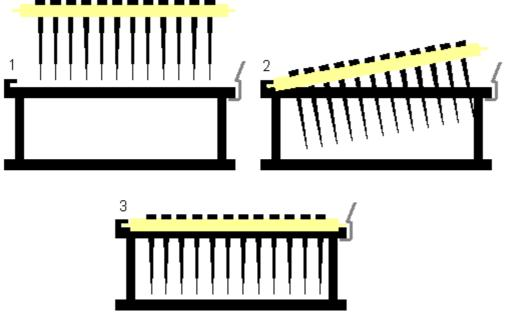
Inserting tips into tip rack holder.
