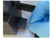
2. Remove the tip ejector by carefully pulling the tip chute upwards.
