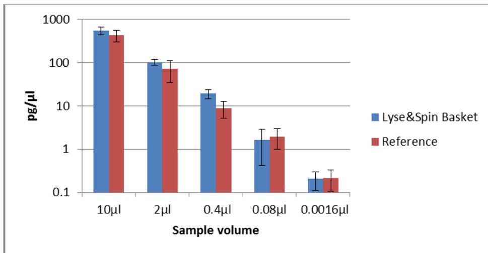
**Figure 3. Sensitivity and linearity with dilutions of blood.** Samples were diluted, and 50 μl containing the stated amount of blood was applied to swabs in 4 replicates each.
