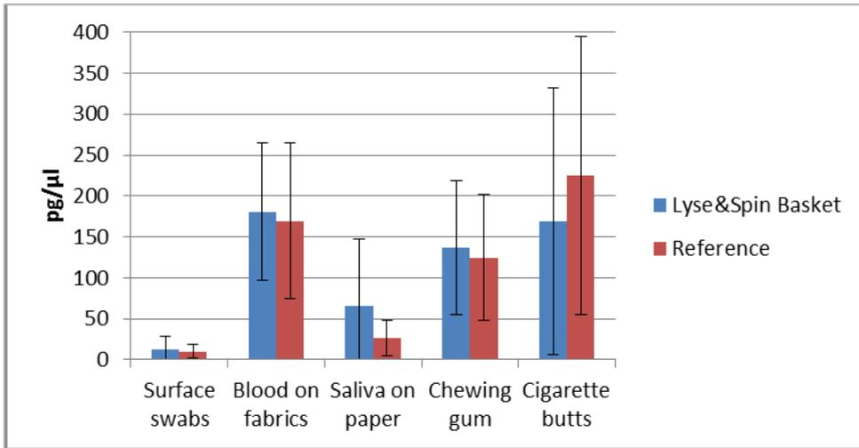
**Figure 8. Various mock casework samples.** 12 samples each were processed using the Investigator Lyse&Spin Basket Kit or the reference method. Samples were extracted on the EZ1 Advanced XL.
