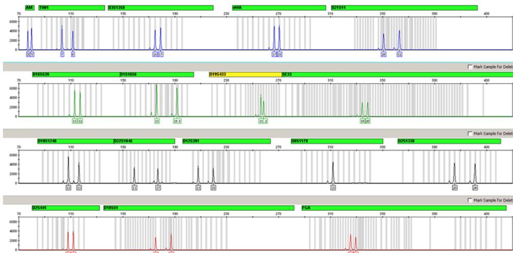
**Figure 9. Example electropherogram of a blood sample on fabric.** 500 pg template DNA was used for amplification.
