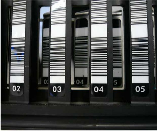
Example of insert for tube carrier.
