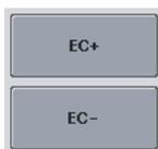
3. Press **EC+** or **EC-** to change the sample type from "Sample" to positive extraction control (EC+) or negative extraction control (EC-).
