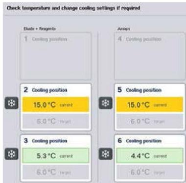
2. To switch cooling off again, press the snowflake button to the left of the cooling position to be switched off.
