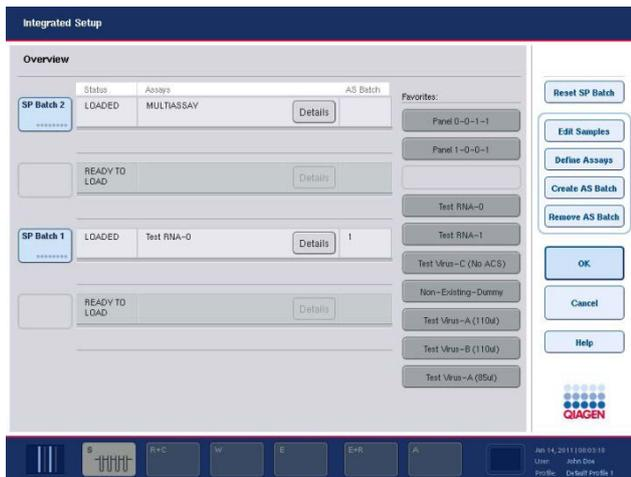
An integrated run consists of one or more integrated batches. An integrated batch is a combination of one or more SP batches and one AS batch. Hence, the eluates of several SP batches can be processed in one AS batch.
