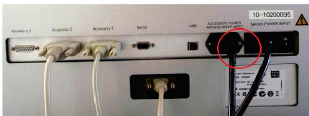
Cables attached to the accessory panel.
