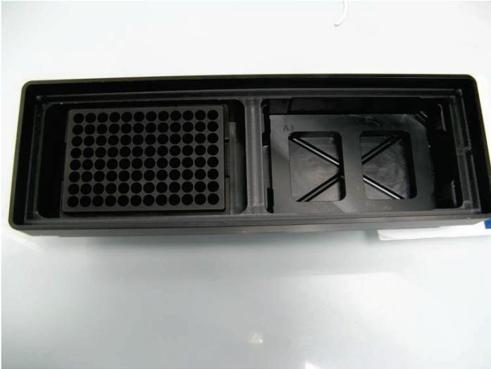
Channelling adapter and riser block EMTR inserted into the vacuum chamber.
