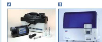
Figure 4. Tissue disruption and genomic DNA purification. (A) The 6770 Freezer/Mill is designed to release DNA from tough biological materials, such as teeth, bone, and skin. (B) The QIAcube automates nucleic acid purification using QIAGEN spin-column kits, standardizing all steps from sample lysis to nucleic acid elution. Up to 12 samples are processed per run.
