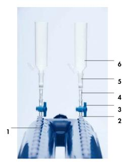
Figure 4. Setting up the QIAvac 24 Plus with QIAamp Mini columns using VacValves, VacConnectors and Tube Extenders. (1: QIAvac 24 Plus vacuum manifold, 2: Luer slot of the QIAvac 24 Plus (closed with luer plug), 3: QIAamp Mini column, 4: VacConnector, VacValve (must be purchased separately), 6: Tube Extender).
