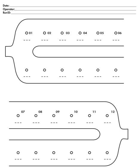
Figure 5. Labeling scheme for tubes and QIA amp Mini columns for use on the QIA vac 24 Plus vacuum system.
