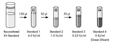
Figure 1. Preparation of standard curve dilution series.
