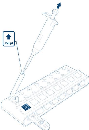
7. Add 150 µl of plasma to the QIArearch QFT Processing Tube containing the QIArearch QFT Diluent Buffer.
