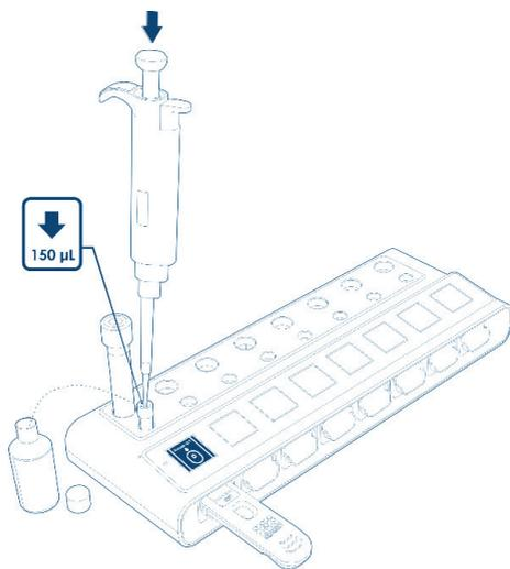
6. Remove the cap from the BCT and set aside. Carefully, remove 150 µL of plasma from the BCT.
