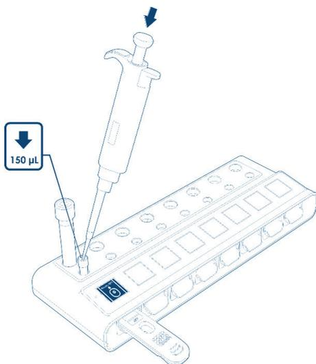
8. Mix the contents of the QIArearch QFT Processing Tube by pipetting up and down at least 4 times. Take care to not introduce foam while pipetting.
