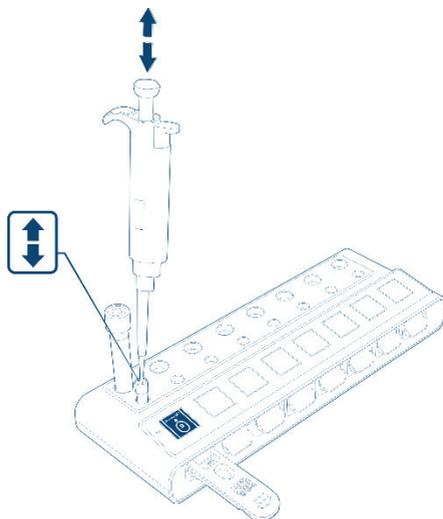
9. Remove 150 µl of sample from the QIArearch QFT Processing Tube and dispense into the sample port of the inserted eStick.
