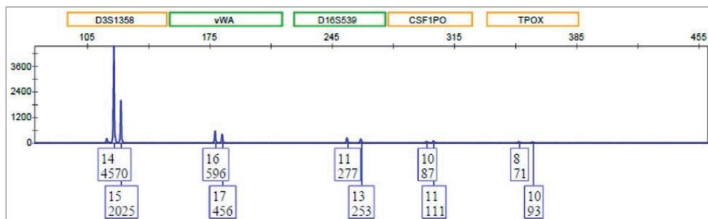
**Figure 2.** Degradation of DNA with added detergent is shown by a decline in signal for larger loci and alleles. Representative electropherogram result of FAM™ dye channel from sample 615707A2 (demineralized with 1% detergent; Degradation Threshold = 126.48). Sample was normalized to 1 ng per PCR, amplified with the GlobalFiler PCR Amplification Kit, typed with the SeqStudio Genetic Analyzer System instrument, and analyzed with GeneMapper ID-X software v1.6.
