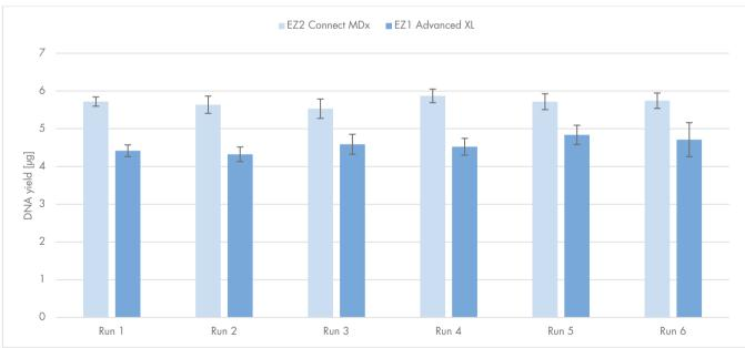
Figure 7. Intra-run precision using the EZ1 DSP DNA Blood system. Blood was collected from a healthy donor in BD K2E tubes and pooled before use. Genomic DNA was purified from 200 µl aliquots in 6 runs of 14 replicates each on the EZ1 Advanced XL, and from 200 µl aliquots in 6 runs of 24 replicates each on the EZ2 Connect MDx using the EZ1 DSP DNA Blood system. Mean total DNA yield and standard deviation are shown for each run.
