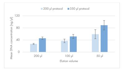
Figure 6. Mean DNA concentration obtained with different elution volumes. Whole blood was collected from 3 donors. Genomic DNA was purified from 200 and 350 µl of each sample and eluted in 200, 100, and 50 µl, each in triplicate, using the EZ1 DSP DNA Blood system on the EZ1 Advanced XL. Mean DNA concentration is shown for each protocol and elution volume.
