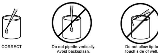
Diagram 1. Correct pipetting.
