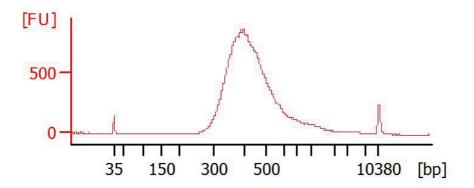
Figure 3. Sample Bioanalyzer image of a GeneRead QIAact Lung DNA UMI library. The majority of the library fragments are between 200–800 bp in size.
