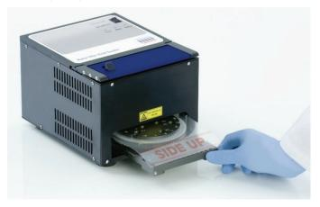
8. To activate the sealing mechanism, first press down on the blue anodized bar at the top of the Heat Sealer, and then push back the black catch.
