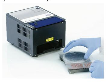
7. Slide the assembly into the Rotor-Disc Heat Sealer using the guide rails on the side of the Rotor-Disc Loading Block. Ensure that the Rotor-Disc Loading Block is pushed in completely.
