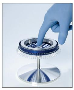
Insert the assembly into the Rotor-Gene Q MDx chamber by clicking into place using the locating pin on the rotor hub. To remove, simply push down on the rotor hub to release and pull out.
