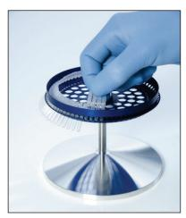
**IMPORTANT**: To achieve maximum temperature uniformity, each position in the rotor must contain a tube. Filling all positions in the rotor ensures even airflow to every tube. Keep a set of empty capped tubes available that can be used to fill any unused positions.
