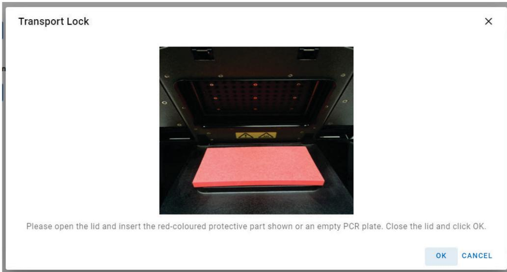
The transport lock is automatically released upon device initialization or switching on the instrument. In case the transport lock should be deactivated without re-starting the instrument, press the **Unlock** button.
