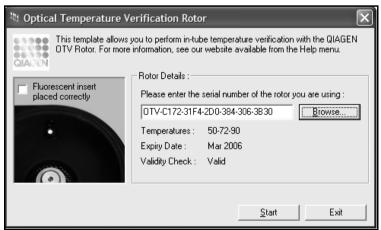
5. The software then prompts for a filename and location to save the run file. Then the run begins. The run performs a series of melts that determine the thermal characteristics of the Rotor-Gene cycler.
