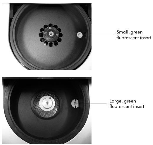
2. Place the OTV Rotor-Disc into a Rotor-Disc 72 Rotor. Secure using a Rotor-Disc 72 Locking Ring. Place the assembly into the Rotor-Gene cycler and click into place. Close the Rotor-Gene cycler lid.
