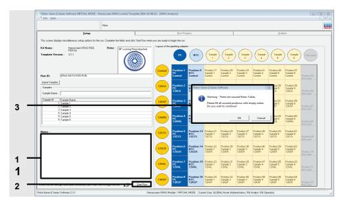
**Note**: If any rotor position is unused, a warning will appear (3 above and 1 in example below) to remind the user that all unused positions on the rotor must be filled with a capped, empty tube.
