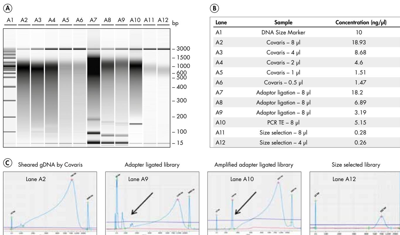
**Figure 5. MiSeq NGS library preparation steps analyzed on the QIAxcel Advanced system. A** Gel image of library samples along the library preparation steps. **B** Sample information table. **C** Single electropherogram view of samples in lanes A2, A9, A10 and A12. Black arrows indicate presence of adapters and primer dimers in the samples after ligation and amplification.
