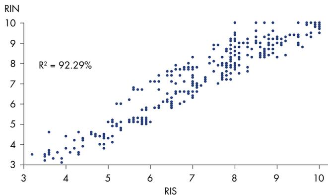
**Figure 4. Correlation of RIN and RIS.** RNA sample purified from rat liver and subjected to a gradient of heat-mediated degradation was analyzed on both the Agilent BioAnalyzer 2100 and the QIAxcel Advanced instrument. The correlation of RIN and RIS values of heat-degraded RNA samples was plotted.
