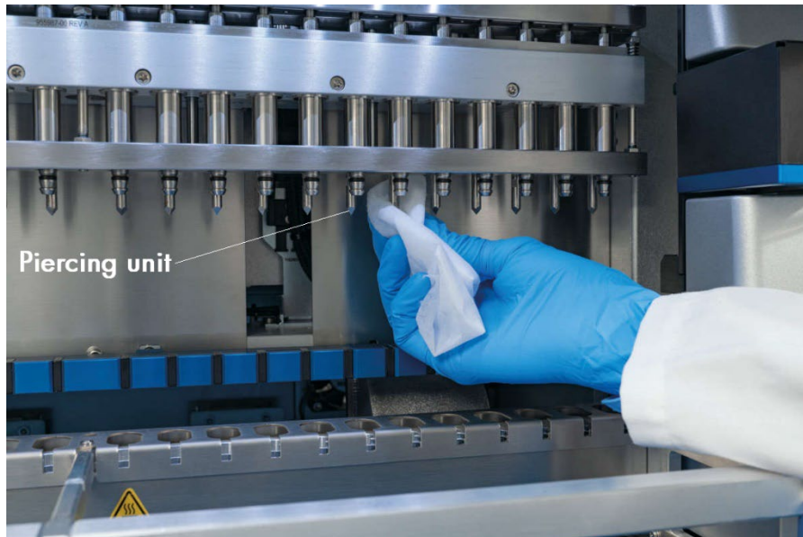
Figure 174. Cleaning the EZ2 piercing unit.
