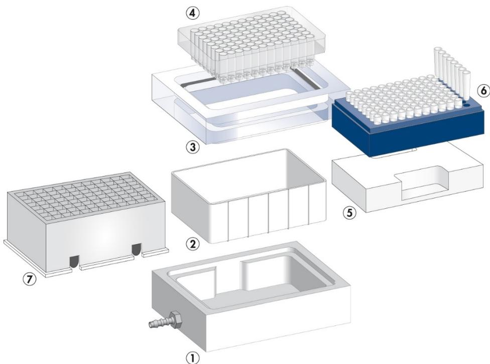
**Figure 3. Components of the QIAvac 96 vacuum manifold.**
