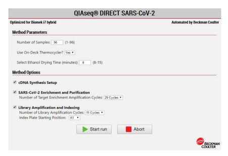
Figure 3. QIAseq® DIRECT enhanced SARS-CoV-2 automated Method Option Selector (MOS) enables users to select sample number, On- or Off-Deck Thermocycler, Ethanol drying time, and method options for index locations and amplification cycles.
