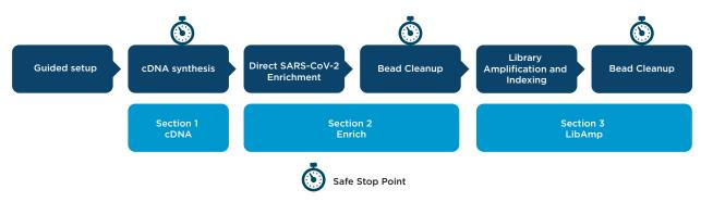
Figure 1. QIAseq® DIRECT enhanced SARS-CoV-2 automated workflow for the Biomek i7 Hybrid Automated Workstation System.
