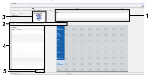
**Figure 3.** Entering the operator name, sample ID, run ID, and "Locking Ring Attached" box. 1 = "Notes" dialog field for operator name, 2 = "Run ID" dialog field, 3 = Checked "Locking Ring Attached" box, 4 = "Sample Name" dialog field, 5 = "Start Run button".
