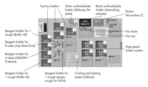
Figure 2. Overview of the BioRobot Universal System worktable.
