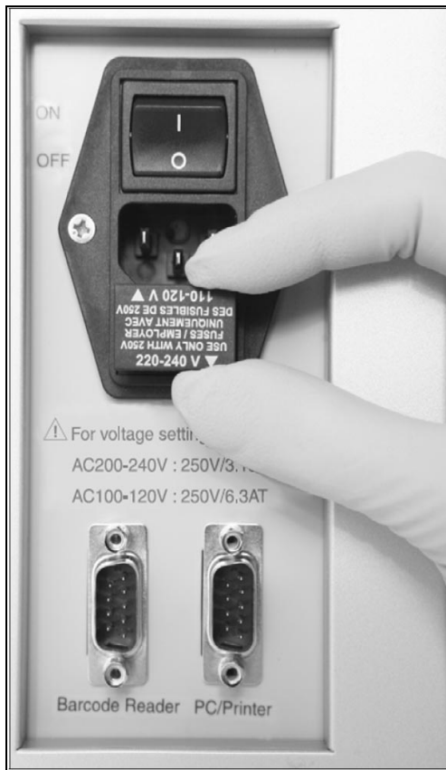
Selecting the correct fuse for 200–240 V line power supply.
