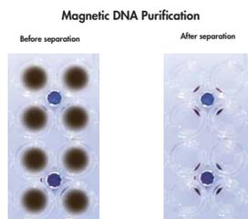
Figure 1 Genomic DNA selectively binds to the surface of the MagAttract particles and can then be further purified by washing the magnetic particles. Magnetic rods, which fit between the wells of a microplate or round well block are used to attract all the particles to one side of the well, allowing the buffer to be removed.
