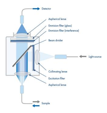
Figure 2. Schematic structure of the epifluorescence spectrometer.
