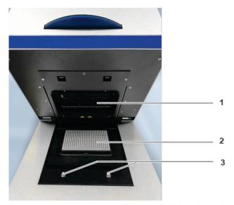
Figure 3. QIAquant 384, open. 1: Heated lid, 2: sample block, and 3: twist locks.
