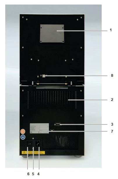
Figure 4. QIAquant 384 rear view. 1: Ventilation for fluorescence spectrometer, 2: ventilation grille for the thermal cycler, 3: service connection, 4: mains connection, 5: fuse holder for instrument fuses, 6: mains switch, 7: type plate, and 8: USB port for PC connection.
