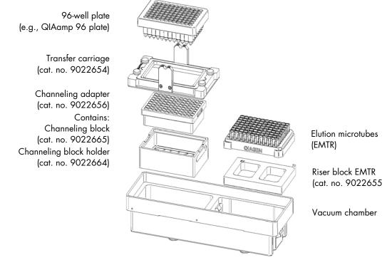
Figure 1. Assembling the vacuum chamber.
