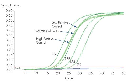
Figure 3. Detection of ABL1 with controls and standards SP3, SP4, SP5, and SP6.  $10^3$ ,  $10^4$ ,  $10^5$ , and  $10^6$  copies/reaction.
