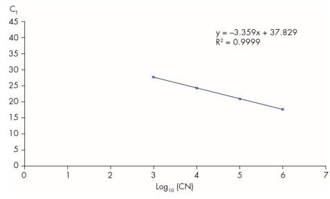
Figure 5. Standard curve for ABL1 calculated from 4 standard dilutions. A linear regression curve (y = ax + b) is calculated, where "a" is the slope of the line and "b" is the y-intercept, which is the y-coordinate of the point where the line crosses the y axis. The equation and coefficient of determination ( $R^2$ ) are shown on the graph.
