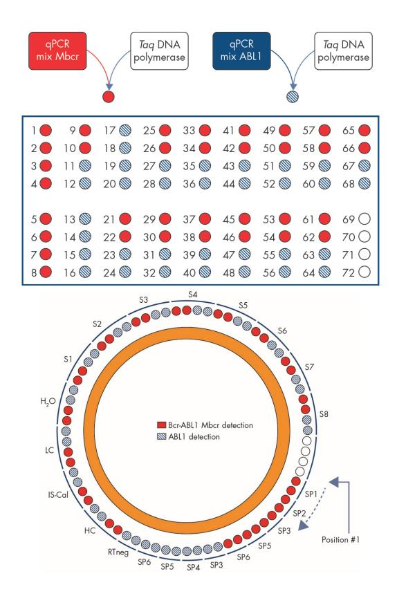
**Figure 2. Rotor setup for each experiment. SP1–SP6**: BCR-ABL1 Mbcr and ABL1 standards; **HC**: High Positive Control; **LC**: Low Positive Control; **IS-Cal**: IS-MMR calibrator; **RTneg**: RT negative control; **S1-S8**: cDNA samples; **H**<sub>2</sub>**O**: water control.
