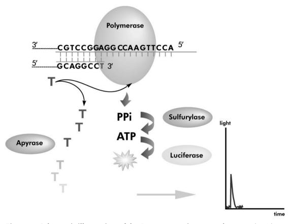
**Figure 1. Schematic illustration of the Pyrosequencing cascade.** As nucleotides are incorporated into the analyzed DNA strand, pyrophosphate is released and converted to ATP. Generated ATP drives the light reaction detected as a peak on the Pyrogram. Apyrase degrades any unincorporated nucleotides.
