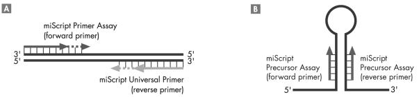
**Figure 8. PCR amplification of mature and precursor miRNA.** A Mature miRNA is quantified using a miScript Primer Assay and the miScript Universal Primer, resulting in a PCR product of 85–87 base pairs. Precursor miRNA is quantified using a miScript Precursor Assay resulting in a PCR product of 45–100 base pairs, depending on the size of the stem-loop.
