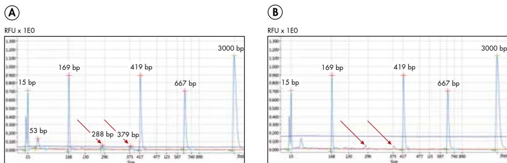
**Figure 4. A The threshold is used during peak detection.** Signals that exceed the threshold value (dark blue line) are detected as peaks. **B** If non-relevant peaks are identified, the threshold can be increased (e.g., to 5 %) to exclude the non-relevant or unspecific data from the analysis.
