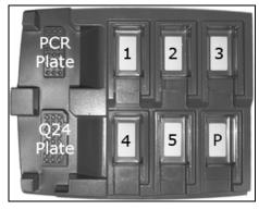
Figure 5. Placement of PCR plate (or strips) and PyroMark Q24 Plate on the PyroMark Q24 MDx Vacuum Workstation. The marked positions contain 70% ethanol (1), PyroMark Denaturation Solution (2), PyroMark Wash Buffer (3), and high-purity water (4, 5). P: Parking position.
