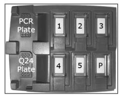
Figure 12. Positions on the PyroMark Q24 MDx Vacuum Workstation.
