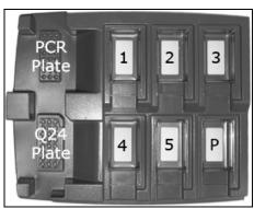
Figure 9. Placement of PCR plate (or strips) and PyroMark Q24 Plate on the PyroMark Q24 MDx Vacuum Workstation. The marked positions contain 70% ethanol (1), PyroMark Denaturation Solution (2), PyroMark Wash Buffer (3), and high-purity water (4, 5). P: Parking position.
