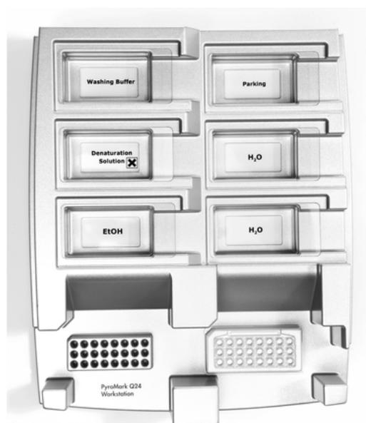
**Figure 3. Placement of PCR plate (or strips) and PyroMark Q24 plate on the vacuum workstation.**
