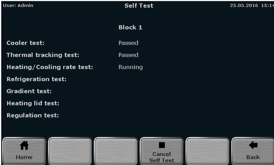
Figure 62. QIAmplifier 96 extended self-test overview screen.
