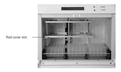
Insert a 5-rod cover into a rod cover slot so that the short tab faces inward and the long tab faces outward. 5-rod covers must be inserted so that they click into place.
