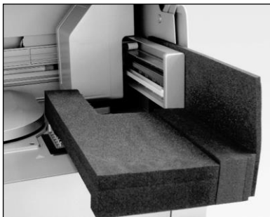
Foam protector for robotic arm.
