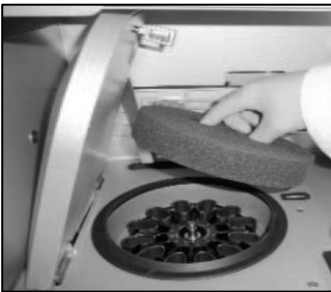
Removing the foam protector from the rotor.
