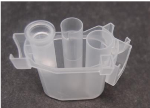
Example of enrichment column loaded into a rotor adapter.
