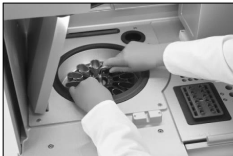
Undoing the rotor nut.
