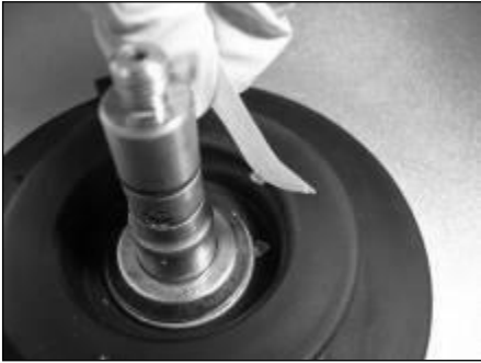
Removing plastic debris with tape.
