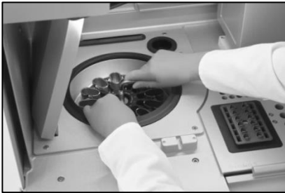
Undoing the rotor nut.
