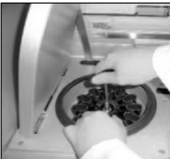
Tightening the rotor using the rotor key.
