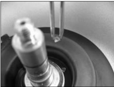
Removing plastic debris with tweezers.
