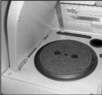
Foam protector for safe transportation of the rotor.
