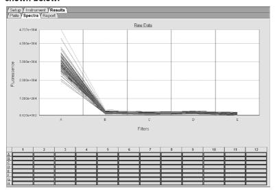
**Note:** If one or more wells produce raw spectra that exceed 72,000 FSU, the background plate or the sample block could contain a fluorescent contaminant.
