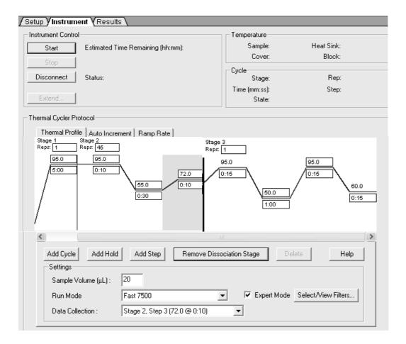
7. Click the "Select/View Filters" dialog field. In the "Filter Selection" box, check only "Filter A" and click "OK".
