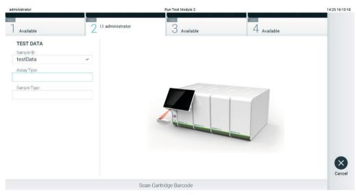
Figure 24. Scanning the QIAstat-Dx assay cartridge bar code.
