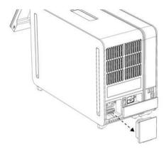
Figure 12. Removing the Termination Bridge.
