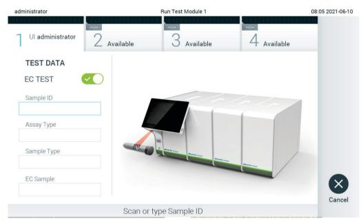
Figure 88. Turning on the EC Test toggle button to enable an EC test.
