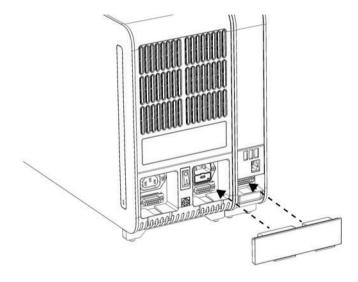
Figure 8. Connecting the Analytical/Operational Module Bridge.
