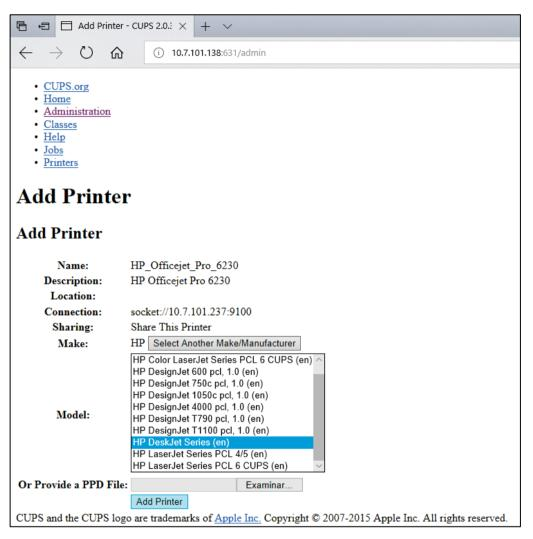
Figure 102. Selecting the printer driver.
