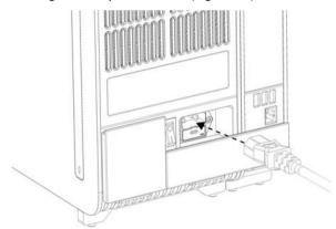
Figure 20. Connecting the power cord.
