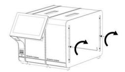
Figure 16. Aligning and attaching the additional Analytical Module.
