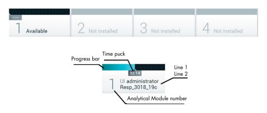
Figure 43. Module status bar.
