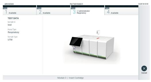
Figure 27. Inserting QIAstat-Dx assay cartridge into QIAstat-Dx Analyzer 1.0.
