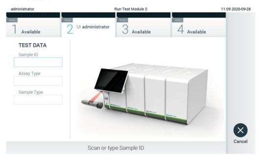
Figure 81. Scanning the sample ID bar code.
