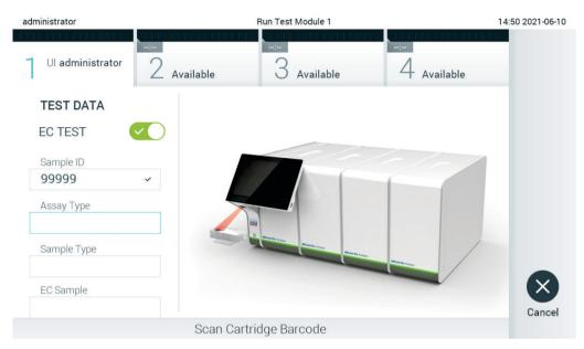
Figure 89. Scanning the QIAstat-Dx assay cartridge bar code.
