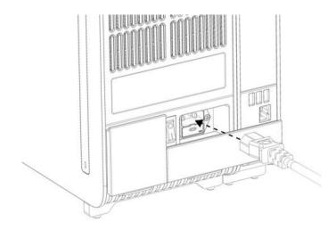
Figure 10. Connecting the power cord.
