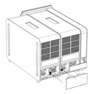
Figure 18. Connecting the Analytical/Analytical Module Bridge.
