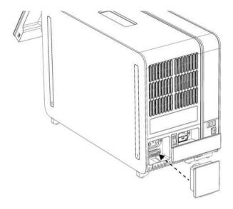
Figure 9. Connecting the Termination Bridge.
