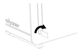
Figure 5. Removing protective covers.
