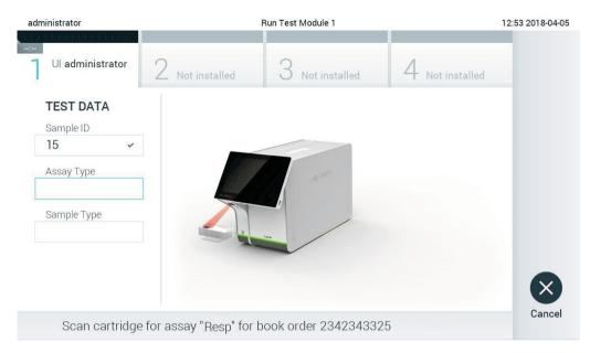
Figure 83. Scanning the QIAstat-Dx assay cartridge bar code.
