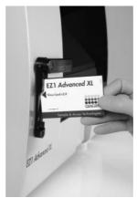
**Figure 2. Ease of protocol setup using EZ1 Cards.** Inserting an EZ1 Card, containing a protocol, into an EZ1 instrument. The instrument should only be switched on after an EZ1 Card is inserted. EZ1 Cards should not be exchanged while the instrument is switched on.
