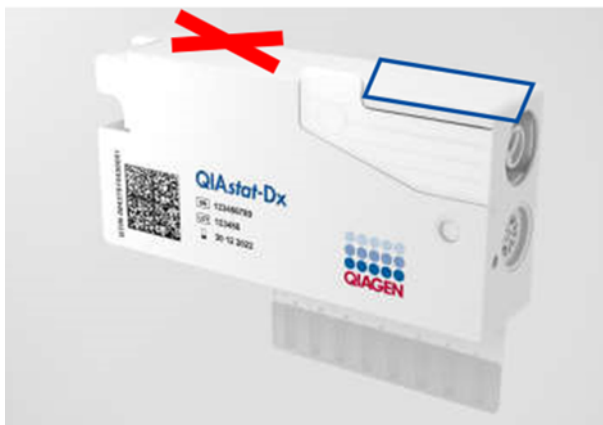
Figure 26. Positioning sample ID barcode.
