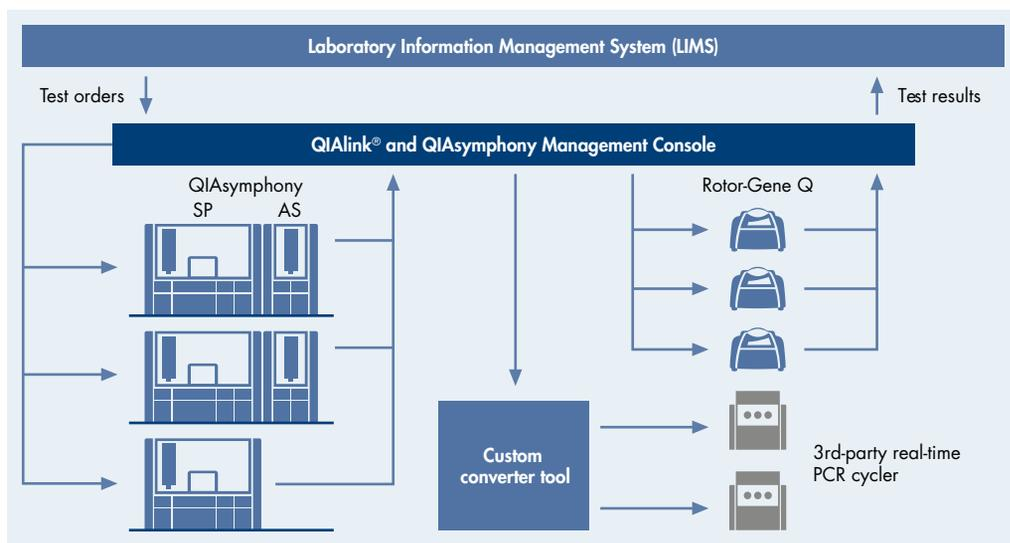
**Figure 3. IT integration at MVZ Labor Dessau (Limbach Group).** Consolidation of instruments results in a lean IT setup, with seamless exchange of test orders and results between the QIAAsymphony RGQ systems and LIMS, and transfer of sample-related data between instruments. Additionally, 3rd-party instruments can be integrated into the system using a custom converter tool.
