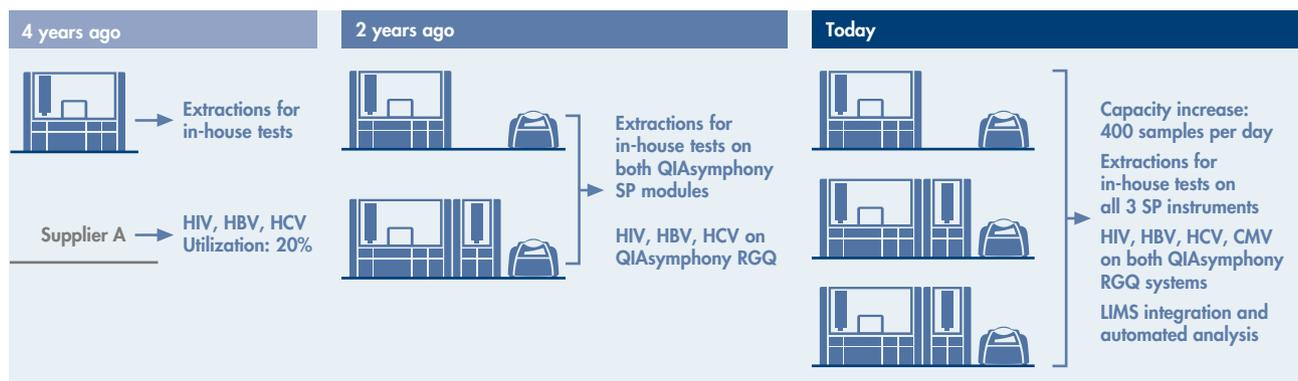
**Figure 1. Workflow optimization and consolidation at MVZ Labor Dessau (Limbach Group).** The laboratory is now able to process up to 400 samples a day on 2 QIAAsymphony RGQ systems and a QIAAsymphony SP instrument plus Rotor-Gene Q cycler. The setup provides increased automation and integration into the Laboratory Information Management System (LIMS), resulting in improved efficiency and cost savings.
